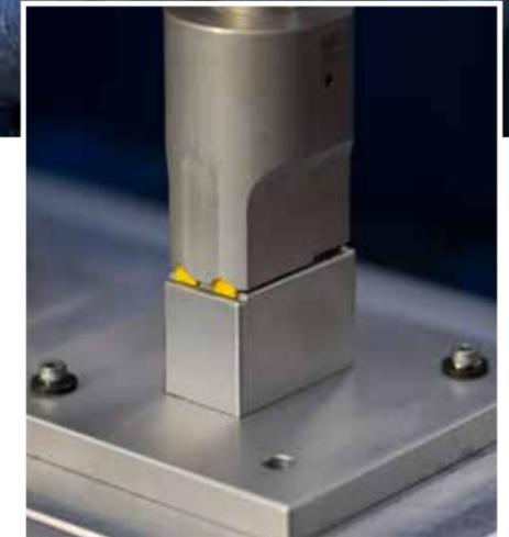
Ultrasonic Welding is a process whereby high frequency vibrations are locally applied to components via a bespoke welding horn. The conversion of electrical to mechanical energy under pressure, creates a friction that melts the plastic at the meeting points. This causes the polymer chains to bond, so that when cooled it creates a solid state weld between components.
